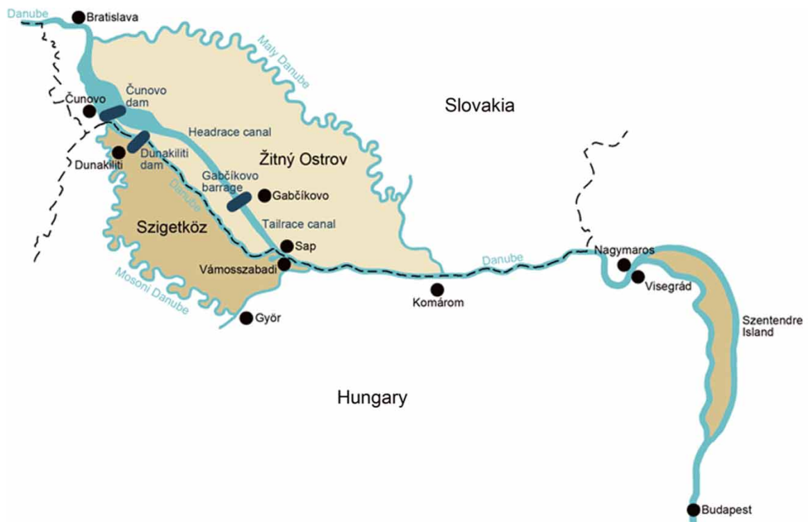
Fig. 2. Sketch of ‘Variant C’. Source: Judgement of the International Court of Justice, p. 25.
